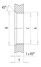
Installation direction: o-ring sits on chamfer.
